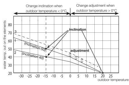
Examples of inclination values for different systems Floor heating onlyindLow temperature system (well-insulated houses)indNormal temperature system (factory setting)indHigh temperature system (older houses, small radiators, poorly insulated)ind
